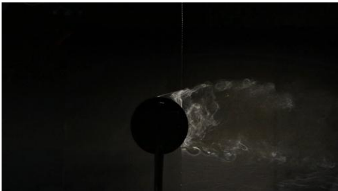
Figure 16 Flow visualization behind a smooth cylinder at the lowest wind speed
