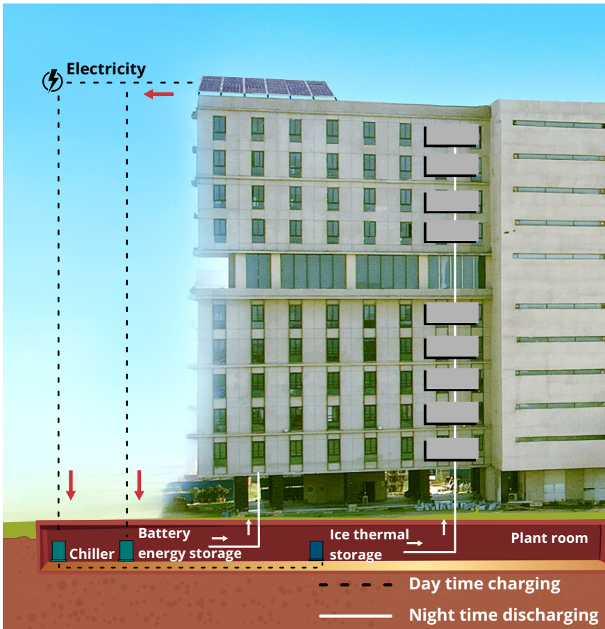
Figure 16 Schematic of thermal storage system
